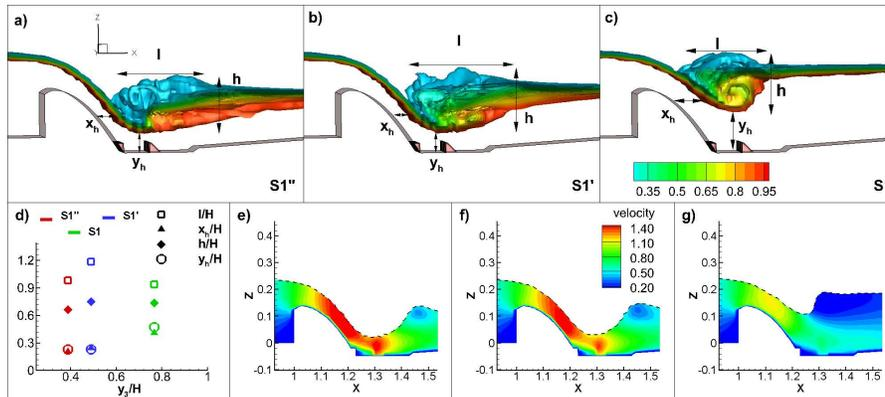
Figure 4: Tail water depth effect in the free surface profile over the spillway and stilling basin; a) Free surface profile for simulation case  $S1''$ ; b) Free surface profile for simulation case  $S1'$ ; c) Free surface profile for simulation case  $S1$ ; d) Adimensional tail water depth versus adimensional jump's length, height and position; e) Velocity profile for simulation case  $S1''$ ; f) Velocity profile for simulation case  $S1'$ ; g) Velocity profile for simulation case  $S1$ .
