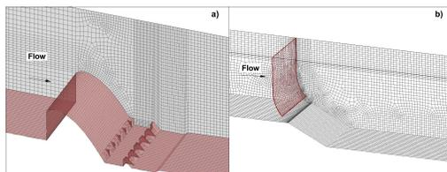
Figure 1: Computational grid used in numerical simulations; a) 3D view of the grid for the spillway and stilling basin;b)3D view of the grid for the gate and dissipation basin.
